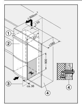
The appliance can be installed in a kitchen run. To match the height of the rest of the kitchen, the appliance can be fitted with a suitable top box 1.
